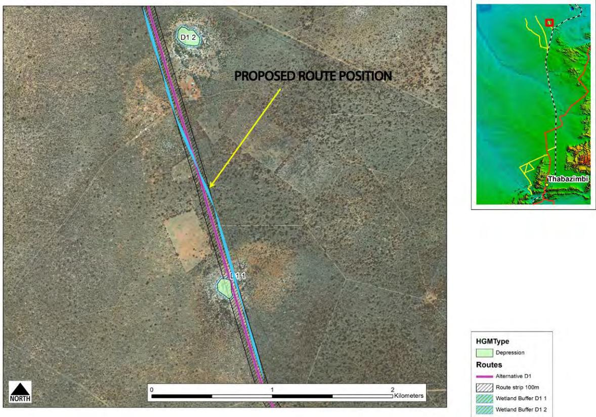
Figure 40. Pipeline placement on Enkeldraai and Taiboshfontein to negate the impact on wetlands D1.1 and D1.2
