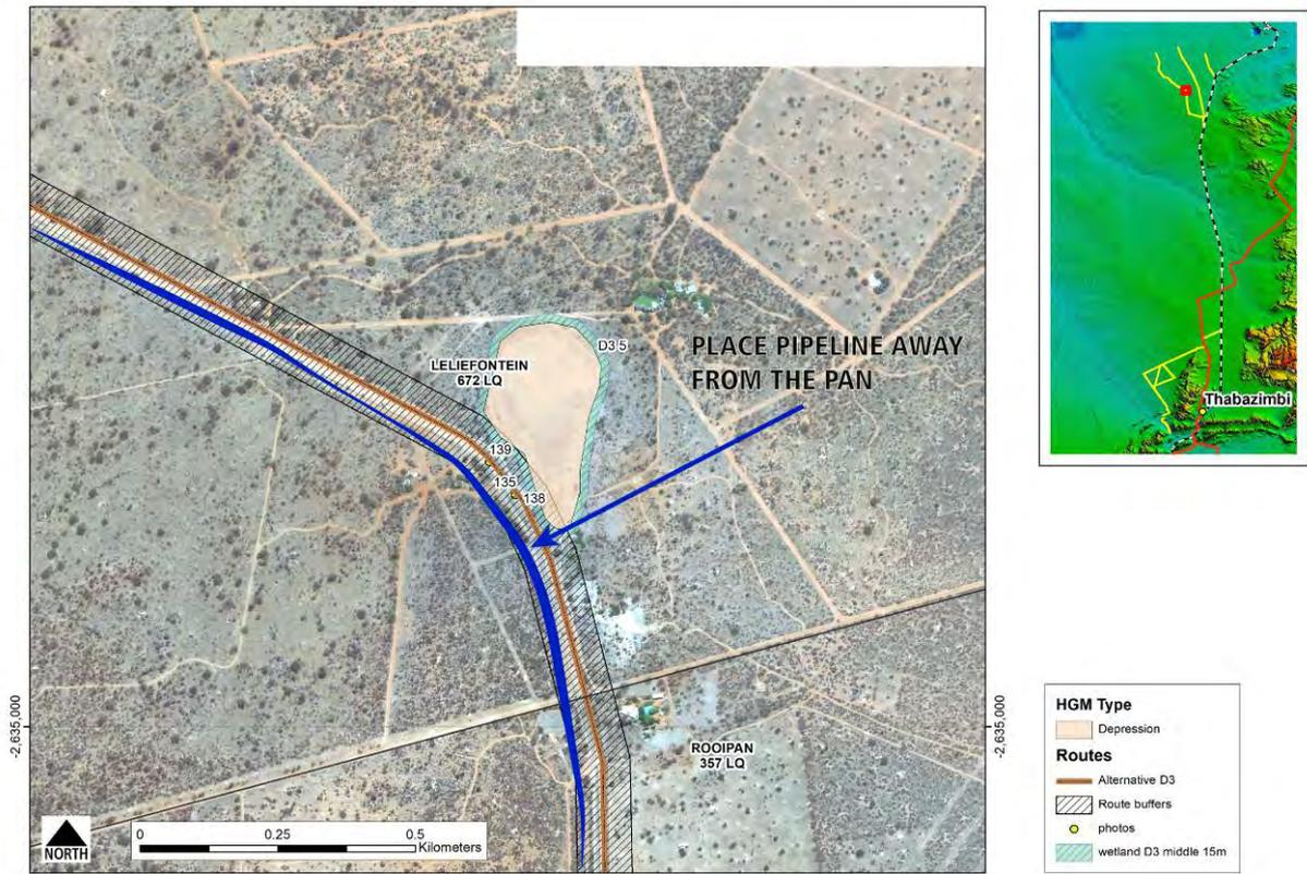
Figure 39. Pipeline placement on Leliefontein to negate the impact on the wetland D3 5
